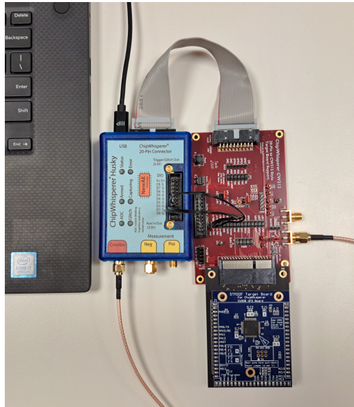
Figure 1: ChipWhisperer-Husky, CW313 adapter board and CW308T-STM32F4 board used in the experiments.
